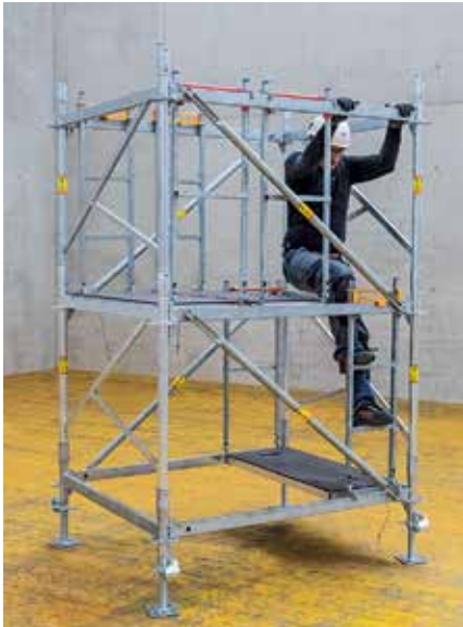
The intermediate guardrail of the Platform MDS can also be used as a climbing aid. The distance is 50 cm on the "red" side and 33 cm on the "yellow" side.
